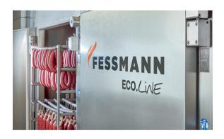
The default package of the T3000 includes an automated cleaning unit; on demand, an additional air conditioning package can be installed for optimised maturing processes.
